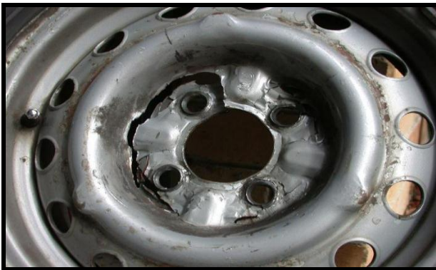
Fig. 1 Crack near the hub hole
