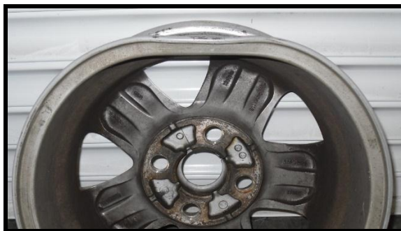
Fig. 2 Bend due to impact:
